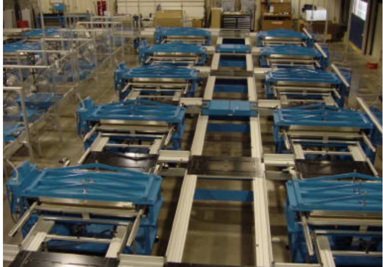
The PowerPallet-equipped production line at Hexcel Manufacturing features semi-autonomous carts exchanging data via wireless DeviceNet.
